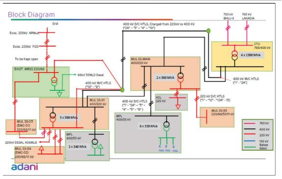
MUL has submitted that in order to cater to the Power Demand of the magnitude as stated above, overall infrastructure plan is developed. In this respect, Petitioner applied to Central Transmission Utility of India Limited (CTUIL) for grant of connectivity at CTU. CTUIL after following due procedure intimated the Grant of Connectivity to Petitioner as Distribution Licensee at 400 kV voltage level Navinal Sub-station proposed (GIS).
