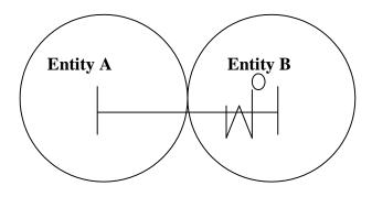
Case- 2: Interconnecting line owned by Entity – B Metering Point: Substation of Entity – A
