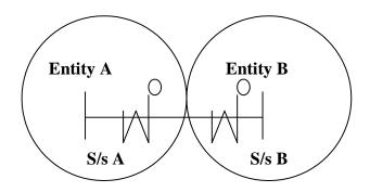
Net VArh exported from S/S-A, while voltage < 97% = X1Net VArh exported from S/S-A, while voltage > 103% = X2Net VArh imported at S/S-B, while voltage < 97% = X3Net VArh imported at S/S-B, while voltage > 103% = X4
